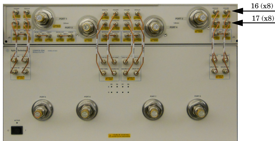
Figure 10 PNA-X RF Interface Cable Connections
